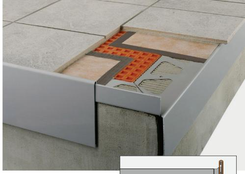
All cavities of the setting material for embedding Schlüter<sup>®</sup>-BARA-RW must be filled to prevent the collection of water, since water with a high alkaline concentration can corrode the aluminium.
