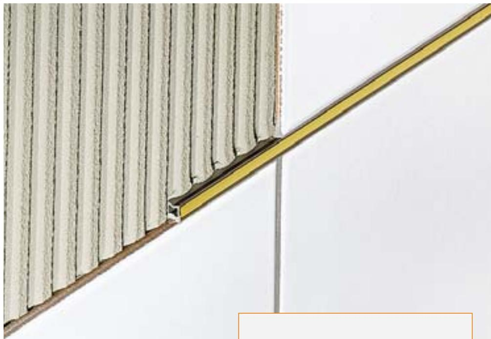
Schlüter®-DILEX-EZ 6 and -EZ 9 are decorative expansion joints used with tiled surfaces. Two soft PVC surfaces connect and overlap rigid PVC side sections at the top and bottom in two different colours, creating two usable surfaces which absorb compressive stresses.
